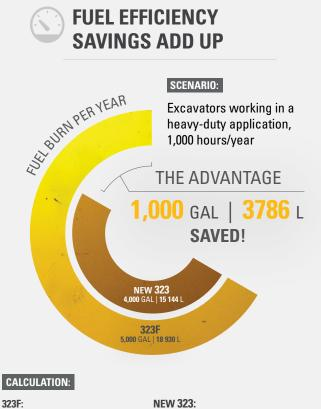
$5.0 \text{ Gal/hr} \times 1,000 \text{ hr/yr} = 5,000 \text{ Gal/yr}$  ( $5.0 \text{ Gal/hr} \times 80\%$ ) x 1,000 hr/yr = 4,000 Gal/yr ( $18.93 \text{ l/hr} \times 1000 \text{ hr/yr} = 18 930 \text{ l/hr}$  ( $18.93 \text{ l/hr} \times 80\%$ ) x 1000 hr/yr = 15 144 l/yr
